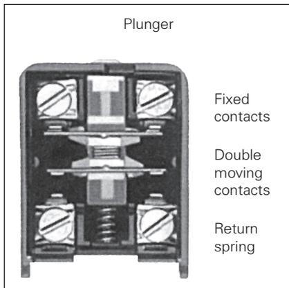
Fig. 4 Slow-action switch with 1 NO + 1NC
