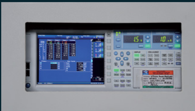
Efficiency determination as per IEC 60034-2-1 : 2024
